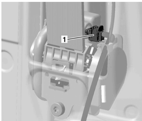
Fig. 1: Automatic belt retractor with pyrotechnical belt tensioner
