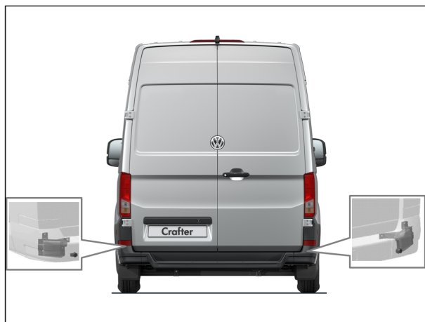
Fig. 1: Position of the radar sensors in the rear bumper
