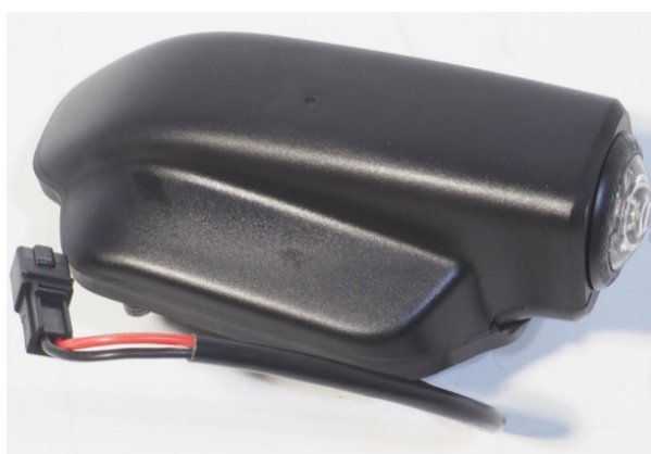
Fig. 3: Right and left side marker lights, part number: 7C0 941 061 C
