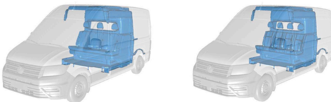
Fig. 1: Schematic diagram of a panel van+ 3-seater bench/4-seater bench conversion in the 2nd seat row.
