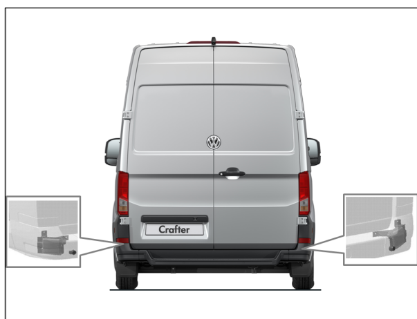
Fig. 3: Position of the radar sensors behind the bumper cover on the left and right
