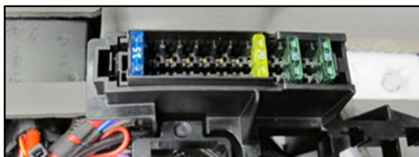
Fig. 3: Detail A: Fuse holder – Connection point for second battery
